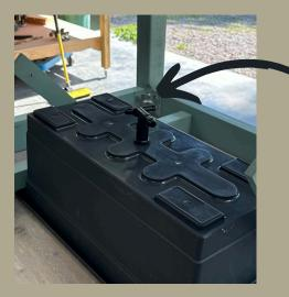
With each tap, insert firmly into the ice trough from the outside and tighten very securely. If the tap isn't tight the joint will leak. Position the taps in the same direction on all the buckets.
